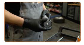
Screw the fixing bolts of the fuel filter bracket. Use Torx T40. Use a ratchet wrench.
