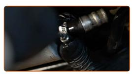
Clean the fuel filter mounting bracket. Use all-purpose cleaning spray.
