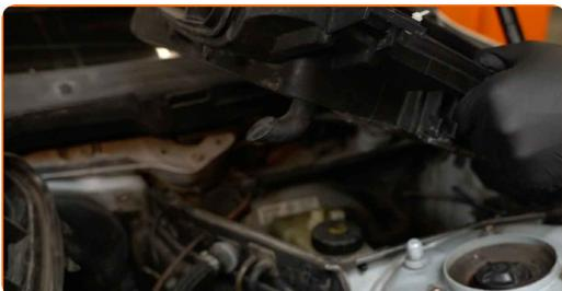
8 Unscrew the brake fluid reservoir cap.
