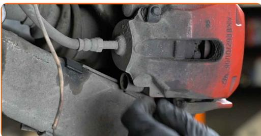
**16** Unscrew the brake caliper fastening. Use HEX No.H7. Use a ratchet wrench.
