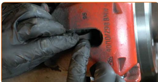
**39** Install the brake caliper retaining spring.
