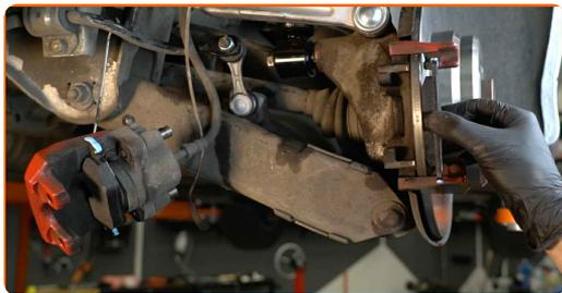
**36** Install the brake caliper and fix it. Use HEX No.H7. Use a torque wrench. Tighten it to 30 Nm torque.
