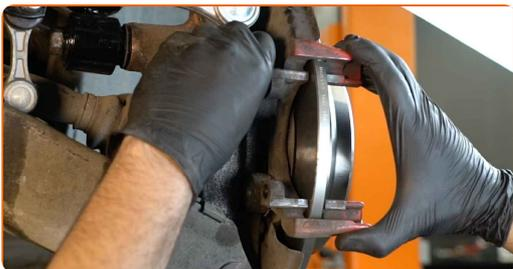
**32** Tighten the brake caliper bracket. Use a drive socket #16. Use a torque wrench. Tighten it to 65 Nm torque.
