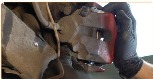
**38** Connect the brake pads wear sensor.
