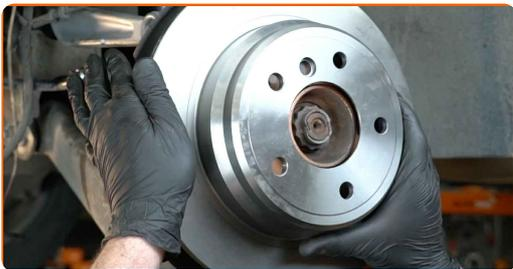
**29** Tighten the brake disc fastening. Use HEX No.H6. Use a torque wrench. Tighten it to 16 Nm torque.
