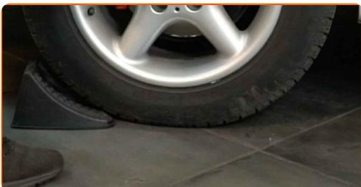
**10** Loosen the wheel mounting bolts. Use wheel impact socket #17.
