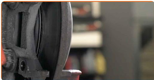
**21** Clean the brake caliper bracket fasteners. Use a wire brush. Use WD-40 spray.
