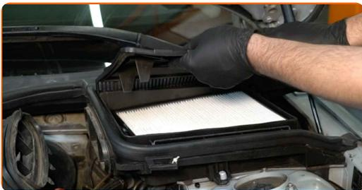
6 Remove the cabin filter housing seal.
