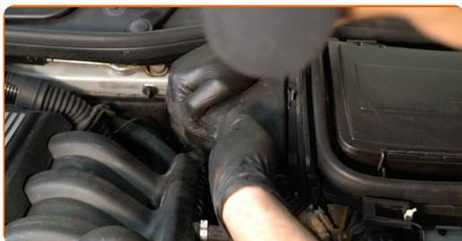
**51** Remove the fender protection cover.
