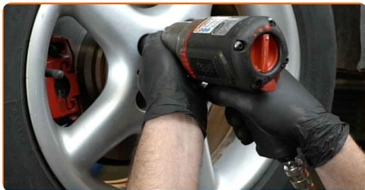
**44** Lower the car and working in a cross order, tighten the wheel bolts. Use wheel impact socket #17. Use a torque wrench. Tighten it to 120 Nm torque.
