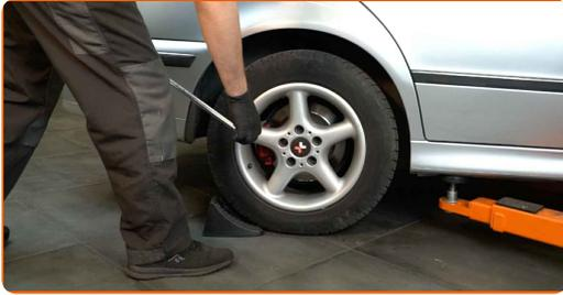
**11** Raise the rear of the car and secure on supports.
