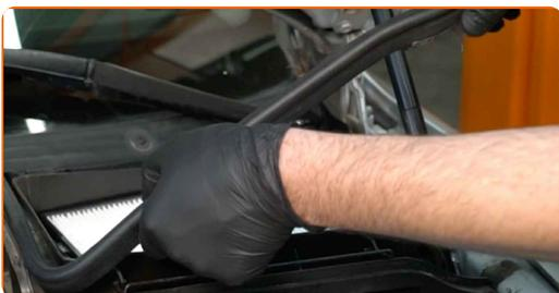
7 Remove the cabin air filter housing.
