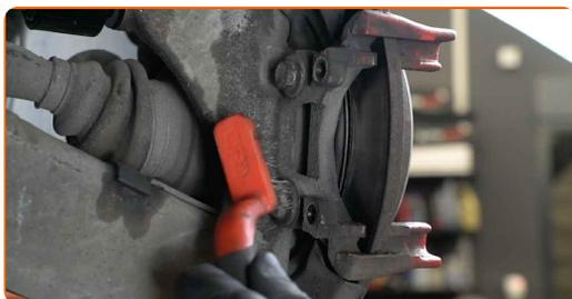
**22** Unscrew the caliper bracket fastening. Use a combination spanner #16.
