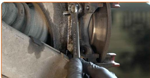
**23** Remove the caliper bracket.
