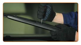
Remove the blade from the wiper arm.
