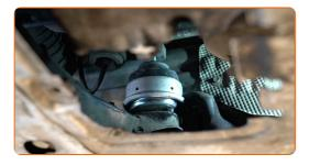
17 Remove the support from under the engine.
