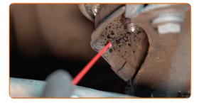
Unscrew the lower fastener of the engine mount. Use a drive socket #16.
