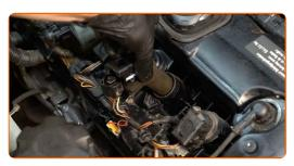
Plug in the ignition coil connector.
