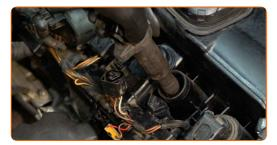
Treat the ignition coil tips. Use high-temperature grease. Use a flat screwdriver.
