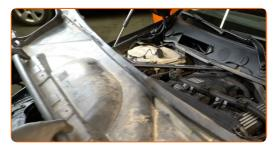
Unscrew the engine cover fastener. Use HEX No.H5. Use a ratchet wrench.
