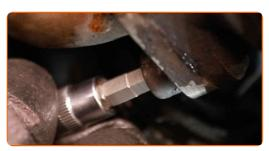
Tighten the EGR cooler fasteners. Use a drive socket #13. Use a torque wrench. Tighten it to 12 Nm torque.
