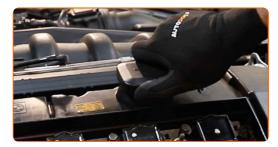
Unplug the connectors from the ignition coils. Use a crowbar.
