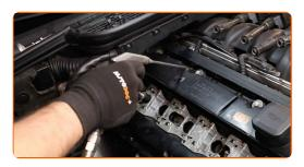
17 Remove the crankcase ventilation hose.
