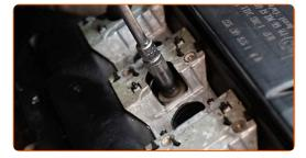
Remove the engine valve cover.
