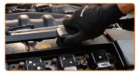
10 Tighten the oil filler cap.
