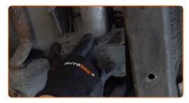
Loosen the clamps of the fuel lines. Use a drive socket #5. Use a ratchet wrench.
