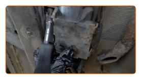
Screw in the fuel pump bracket fastener. Use HEX No.H5. Use a ratchet wrench.
