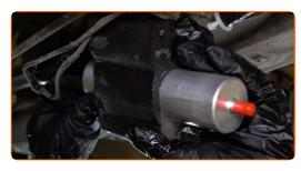
Attach the fuel line to the fuel pump.
