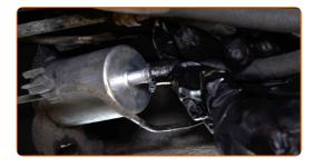
Screw in the clamps of the fuel lines. Use a drive socket #5. Use a ratchet wrench.
