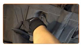
Remove the plastic car body protective cover.
