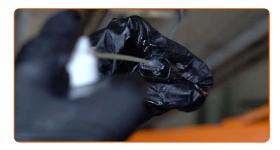
14 Attach the fuel pump connector.
