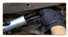
16 Install a new fuel pump into the holder.
