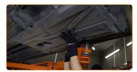
Screw in the fasteners of the plastic car body protective cover. Use a drive socket #8. Use a drive socket #10. Use a Phillips screwdriver. Use a ratchet wrench.
