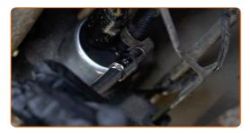
Install the fuel pump together with its holder.
