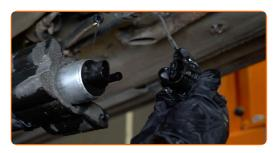
Remove the fuel pump together with its holder.
