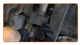
6 Remove the fuel pump bracket.
