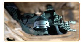
Remove the support from under the engine.
