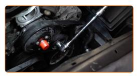
Tighten the water pump pulley fastener. Use a drive socket #10. Use a torque wrench. Tighten it to 17 nm torque.
