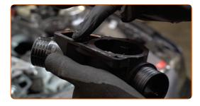
Install the thermostat housing.
