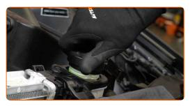
Screw on the coolant reservoir cap.
