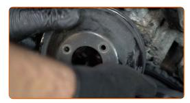
Clean the water pump mounting seat. Use a wire brush. Use all-purpose cleaning spray.
