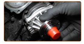
Tighten the water pump fasteners. Use a drive socket #10. Use a torque wrench. Tighten it to 9 nm torque.
