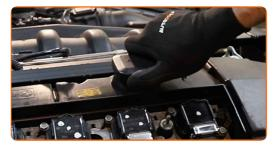
Tighten the oil filler cap.
