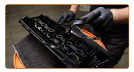
Treat the engine valve cover mounting seat. Use a sealant.
