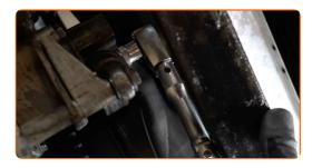
12 Install the AC compressor belt.
