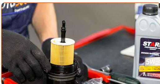
**25** Screw the new filter into its place. Use the 86/16 F socket. Use a torque wrench. Tighten it to 23 Nm torque.
