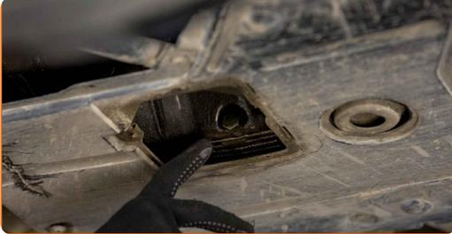
**6** Unscrew the drain plug. Use a drive socket #17. Use a ratchet wrench.
