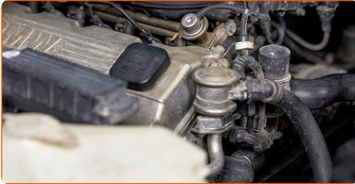
**31** Tighten the oil filler cap.
