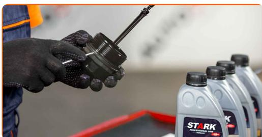
**21** Clean the oil filter housing cap. Use all-purpose cleaning spray.
