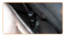
19 Install the air duct housing.
