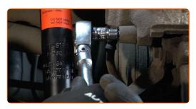
Detach the brake caliper retaining spring. Use a crowbar. Use a flat screwdriver.
