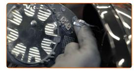
6 Attach the mirror heating connectors.
