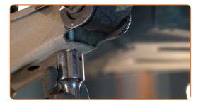
Remove the fastening bolt. Use a pin punch. Use a rubber mallet.
