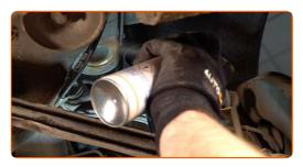
Pull down the suspension control arm. Install the spring.
