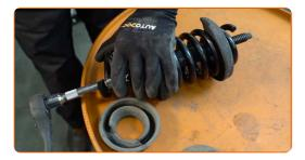
23 Install the rubber spacer on the new coil spring.
