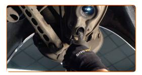
Tighten the fastener connecting the control arm to the rear subframe. Use a combination spanner #18. Use a drive socket #21. Use a torque wrench. Tighten it to 165 nm torque.
