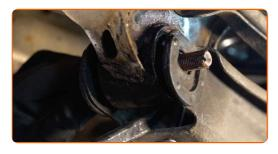
Remove the support from under the arm.
