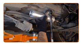
Attach the fuel pressure regulator to the fuel filter. Install the snap ring of the fuel pressure regulator's retainer clip.
