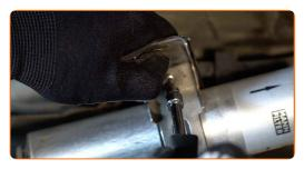
Tighten the fuel filter fasteners. Use a drive socket #13. Use a ratchet wrench.
