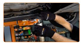
Unscrew the fastener of the fuel filter bracket. Use Torx T20. Use a ratchet wrench.
