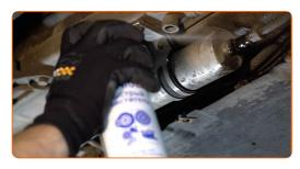
Loosen the fuel filter clamps. Use a flat screwdriver.
