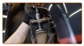
Install the brake caliper and fix it. Use a combination spanner #15. Use a drive socket #13. Use a torque wrench. Tighten it to 35 Nm torque.
