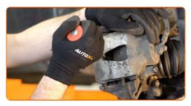
10 Remove the brake caliper.
