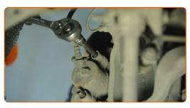
Remove the brake caliper.
