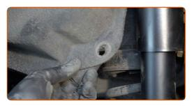
Disconnect the brake pad wear sensor plug.
