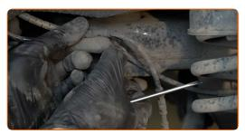
Unscrew the wheel arch cover fasteners. Use a drive socket #10. Use a ratchet wrench.
