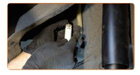
Install the wheel arch cover to its mounting seat. Screw in the fasteners. Use a drive socket #10. Use a ratchet wrench.
