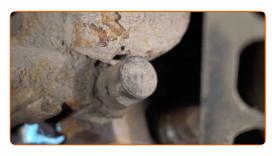
Connect the brake pads wear sensor.
