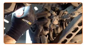
Remove the brake caliper.
