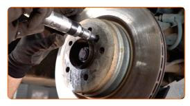
Remove the brake disc.
