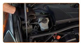
Unscrew the brake fluid reservoir cap.
