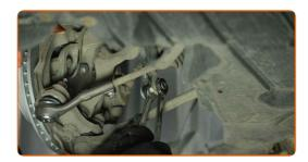
Tighten the fastener connecting the stabilizer link to the shock strut. Use a combination spanner #17. Use a drive socket #16. Use a torque wrench. Tighten it to 58 Nm torque.
