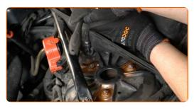
Put the protective caps onto the shock absorber mounting fastener.
