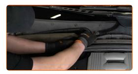
Unscrew the fasteners of the cabin filter housing cover. Use a drive socket #13. Use a ratchet wrench.
