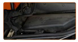
Unscrew the fasteners of the bottom part of the cabin filter housing. Use Torx T25. Use a ratchet wrench.
