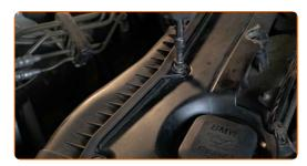
Put the back section of the engine cover back in place.
