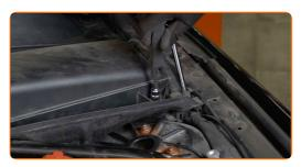
Screw in the fasteners of the bottom part of the cabin filter housing. Use Torx T25. Use a ratchet wrench.
