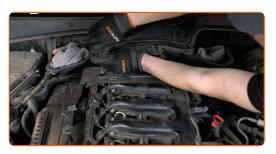
Install the engine cover and secure it.
