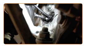
Remove the ABS sensor from the steering knuckle. Use round-nose pliers.
