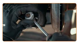
Unscrew the fastener connecting the control arm to the subframe. Use a drive socket #18. Use a crowbar.
