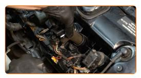
Plug in the ignition coil connector.
