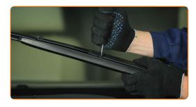
Remove the blade from the wiper arm.
