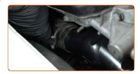
Fasten the clamps of the coolant hoses. Use a drive socket #7. Use a ratchet wrench.
