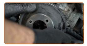
Clean the water pump mounting seat. Use a wire brush. Use all-purpose cleaning spray.
