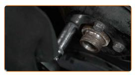
Pull aside the V-ribbed belt tensioner pulley. Use a drive socket #16. Use a ratchet wrench.
