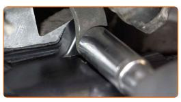
Tighten the thermostat housing fasteners. Use a drive socket #10. Use a torque wrench. Tighten it to 7 nm torque.
