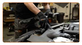
5 Unscrew the coolant reservoir cap.
