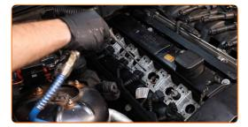
33 Install the ignition coils to the spark plug wells.
