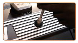
Install the engine cover and secure it.
