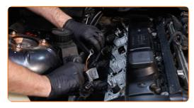
Tighten the chassis (ground) terminal of the ignition coils. Use a drive socket #8. Use a ratchet wrench.
