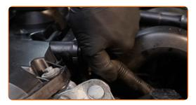
Secure the wiring of the ignition coils in its mounting seats.
