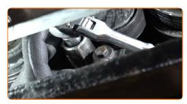
Remove the AC compressor belt.
