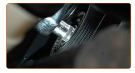
Pull aside the AC compressor belt tensioner pulley. Use a drive socket #13.
