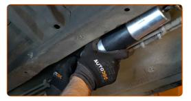
Screw in the fuel filter mounting bracket. Use HEX No.H5. Use a ratchet wrench.
