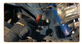
Unscrew the fastener connecting the stabilizer bar with the control arm. Use a combination spanner #13. Use a drive socket #13. Use a ratchet wrench.
