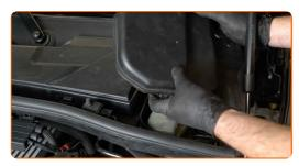
Unscrew the brake fluid reservoir cap.
