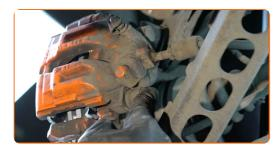
Connect the brake pads wear sensor.
