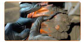
Install the brake caliper retaining spring.
