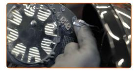
6 Attach the mirror heating connectors.
