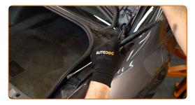
Clean the fasteners of the boot lid gas strut.
