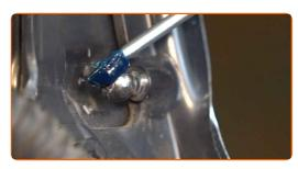
7 Install the new boot lid gas strut.
