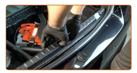
Unscrew the fastener of the boot side lining. Use a clip removal tool. Use Torx T40. Use a ratchet wrench.
