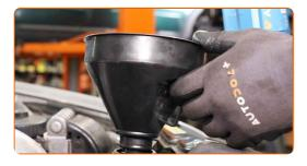
Pour coolant in the coolant reservoir.
