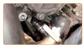
Remove the thermostat housing.
