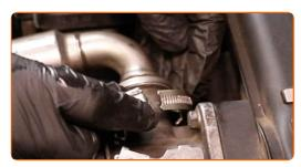
Unscrew the EGR cooler fasteners. Use a combination spanner #13.
