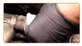
Unscrew the EGR cooler fasteners. Use HEX No.H5.
