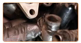
Remove the microfibre cloth from the EGR cooler pipe.
