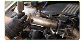
Cover the EGR cooler pipe with a microfibre cloth to prevent dust and dirt from entering the system.
