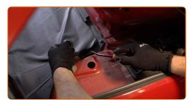
Clean the fasteners of the shock absorber upper mount. Use WD-40 spray.
