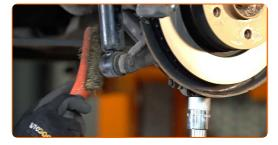
Unscrew the lower fastener of the shock absorber. Use a drive socket #18. Use a tap wrench.
