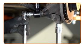
Remove the support from under the arm.
