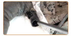
14 Attach the connector of the brake pad wear sensor.
