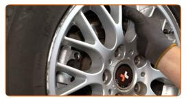
Remove the brake pad wear sensor from the brake pad. Use round-nose pliers.
