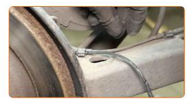
Treat the brake pad wear sensor plug. Use dielectric grease.
