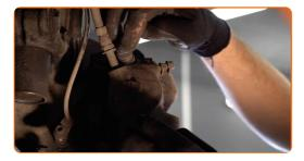
Install the brake caliper retaining spring.
