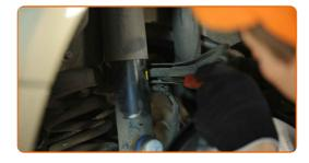
Disconnect the ABS sensor wiring. Use a flat screwdriver.
