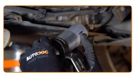
Tighten the fastener of the fuel filter bracket. Use Torx T20. Use a ratchet wrench.
