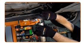
Unscrew the fastener of the fuel filter bracket. Use Torx T20. Use a ratchet wrench.
