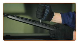
Remove the blade from the wiper arm.
