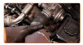
Install the fastening clamps of the air filter breather pipe and the air filter inlet pipe. Use a drive socket #7. Use a ratchet wrench.
