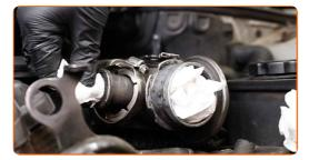
Disconnect the coolant pipe retaining clip. Use a crowbar.
