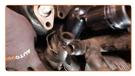
Connect the coolant pipe retaining clip.
