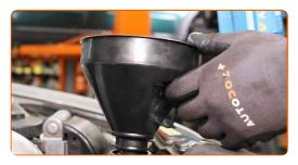
Pour coolant in the coolant reservoir.
