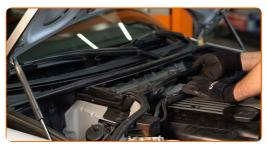
Screw the filter housing fastening bolts. Use Torx T20. Use a ratchet wrench.
