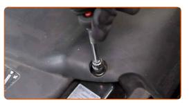
Remove the fender protection cover.
