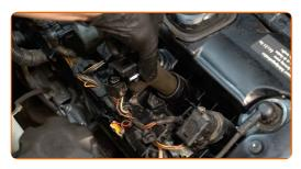
Plug in the ignition coil connector.
