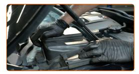
Attach the cable duct to the upper part of the microfilter housing.
