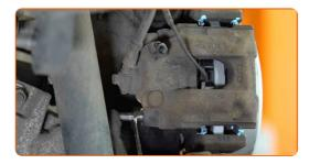
23 Install the dust boot caps of the brake caliper guide pins.
