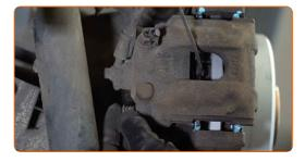
Install the brake caliper retaining spring.
