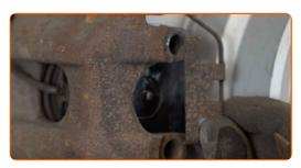
14 Remove the brake caliper.
